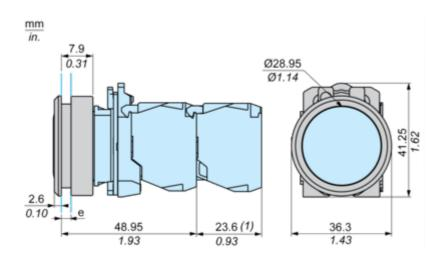
e : Clamping thickness : 1 to 3.5 mm / 0.04 to 0.14 in.(1) Additional row of contacts or double contact
