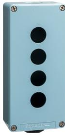
Harmony XAP XB2 SL, Empty control station, zinc alloy, blue, 4 cut-outs, Ø22, with ISO cable entries, 80 x 175 x 51.5 mm
