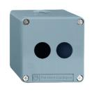
Harmony XAP XB2 SL, Empty control station, zinc alloy, blue, 2 cut-outs, Ø22, with ISO cable entries, 80 x 80 x 51.5 mm
