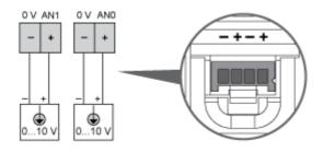
The (-) poles are connected internally.
