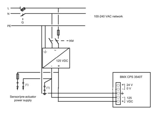
**Q** General isolator **KM** Line contactor or circuit breaker
