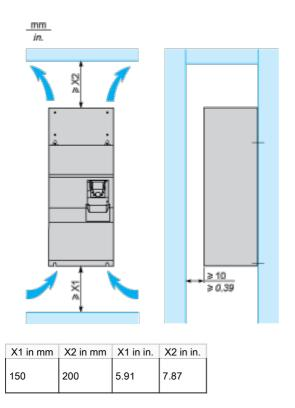
These drives can be mounted side by side, observing the following mounting recommendations:
