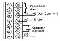
NOTE: A normally closed relay contact rated at 220 Vac, 6A / 30 Vdc, 5A is available on terminals 1 and 2 of the power terminal strip. This contact set may be used to signal input power OFF, or a power supply failure.
